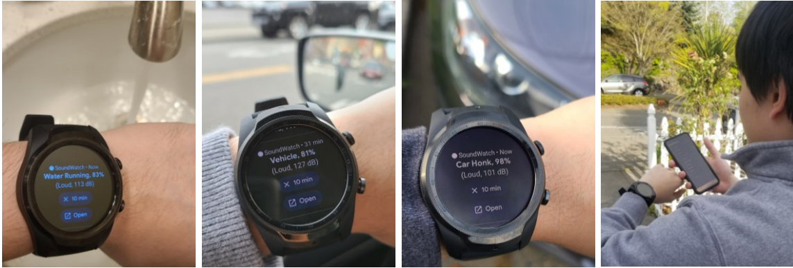
Figure 1: SoundWatch uses a deep-CNN based sound classifier to classify and provide feedback about environmental sounds on a smartwatch in real-time . Images show different use cases of the app and one of the four architectures we built ( watch+phone ).
